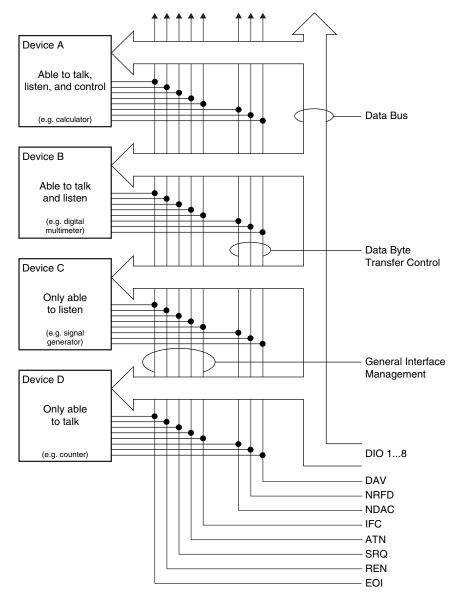
Figure 1—Interface capabilities and bus structure
